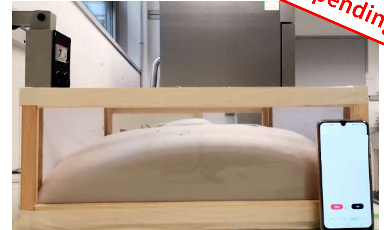
Expansion of FenX foam from waste
